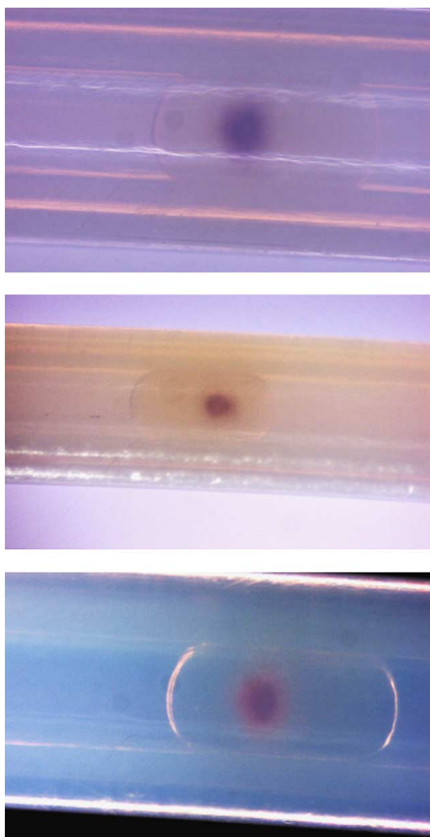
Fig. 26. Three examples of monoclonal cultures obtained in micro fluid segments (inner diameter of tubes 0.5 mm).
